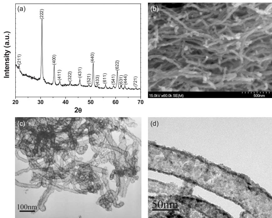
**Figure 3.** Morphological and structural characterizations of regular  $\text{In}_2\text{O}_3$  nanotubes prepared by the calcination of  $\text{In}_2\text{O}_3$ /polyelectrolyte/CNT nanocomposites at 550 °C in  $\text{O}_2$  for 3 h: a) XRD pattern; b) FESEM image; c, d) TEM images.
