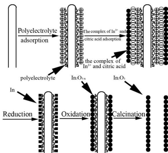
Figure 1. Schematic diagram for the growth process of  $\text{In}_2\text{O}_3$  nanotubes.
