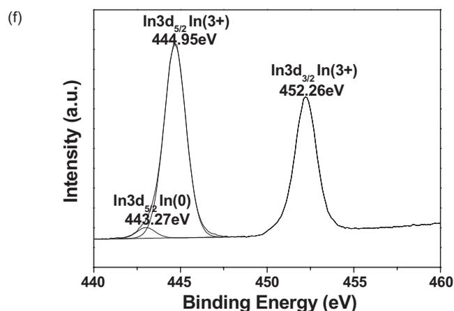
Figure 2. a) TEM image of pure CNTs and b–f) morphological, structural and compositional characterizations of  $\text{In}_2\text{O}_3$ /polyelectrolyte/CNTs nanocomposites prepared by the layer-by-layer assembly and chemical precipitation: b) TEM image, c,d) HRTEM images of an individual CNT, and e,f) XPS spectra.
