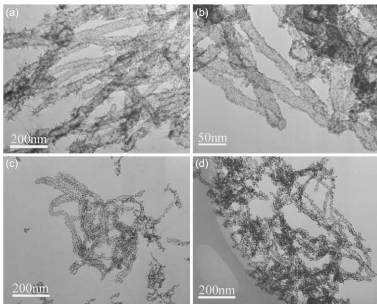
**Figure 4.** TEM images of a) NiO, b)  $\text{SnO}_2$ , c)  $\text{Fe}_2\text{O}_3$ , and d) CuO nanotubes prepared by the LBL-based approach in combination with subsequent calcination.
