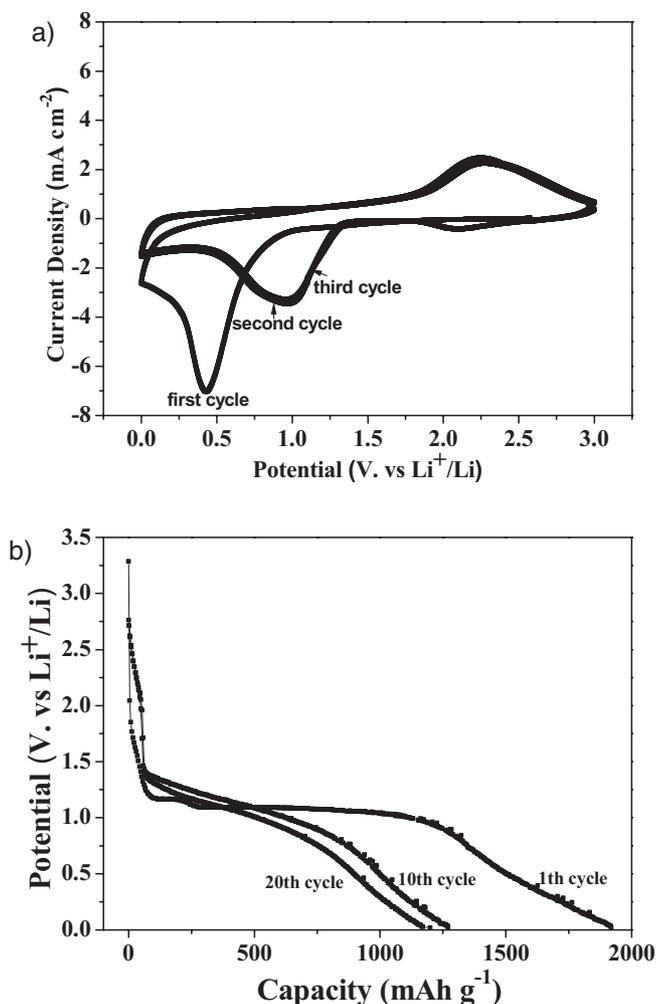
**Figure 3.** The first three CV curves of the porous  $\text{Co}_3\text{O}_4$  nanotube based anode materials at a scan rate of  $0.5 \text{ mVs}^{-1}$  and a temperature of  $20^\circ\text{C}$  (a); The 1st, 10th and 20th discharge curves of the porous  $\text{Co}_3\text{O}_4$  nanotube based anode materials at a current density of  $50 \text{ mA g}^{-1}$  and a temperature of  $20^\circ\text{C}$  (b).
