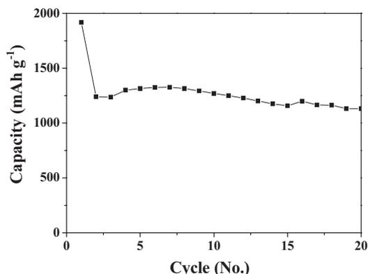
**Figure 4.** Discharge capacity versus cycle number for the porous  $\text{Co}_3\text{O}_4$  nanotube based anode materials at a current density of  $50 \text{ mA g}^{-1}$  and a temperature of  $20^\circ\text{C}$ .
