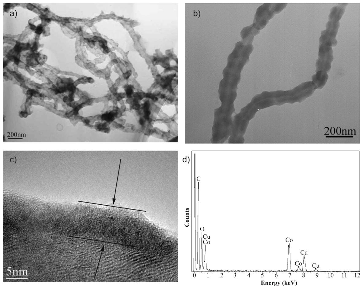
**Figure 1.** Morphological and structural characterizations of CNTs- $\text{CoO}_x$  nanocables prepared by the sonication for 1 h at room temperature in the hexane solution of  $\text{Co}_4(\text{CO})_{12}$  and CNTs: a), b) TEM image; c) HRTEM image; d) EDX pattern.
