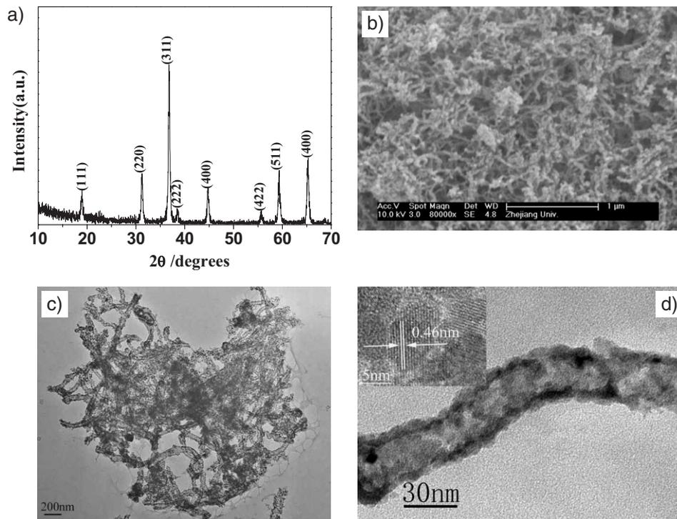
**Figure 2.** Morphological and structural characterizations of the  $\text{Co}_3\text{O}_4$  nanotubes prepared by the calcination of CNT- $\text{Co}_x$  nanocables at  $500^\circ\text{C}$  in  $\text{O}_2$  for 3 h: a) XRD pattern; b) FESEM image; c), d) TEM image. The upper-left inset in d corresponds to the HRTEM image.
