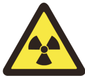
当心电离辐射 Caution, ionizing radiation
